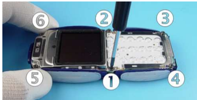
Unscrew the six Torx Plus® size 6 screws. For assembly, the reverse order and a Torx Plus® driver with a torque of 28Ncm has to be used.
