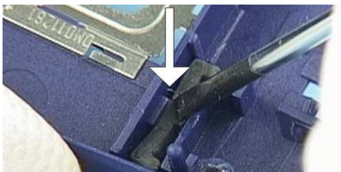
Push out the Blind Plug by using a screwdriver.
