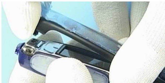
Lift the topside of the A-Cover and then remove it carefully.
