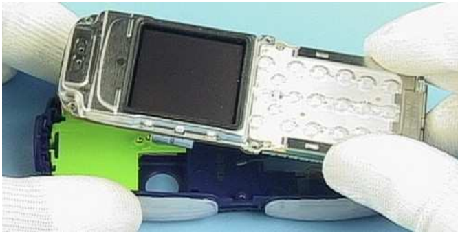
Separate the Modules from B-Cover.
