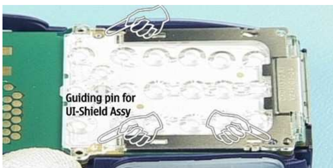
Note the guiding pins when attaching the Light Guide Assy.
