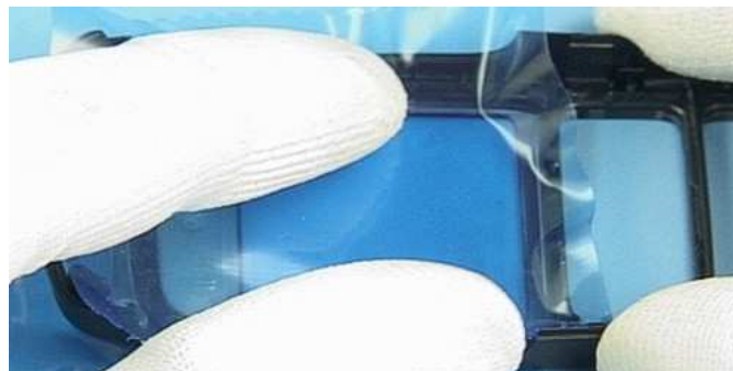
Also protect the inner side of A-Cover with a plastic film.
