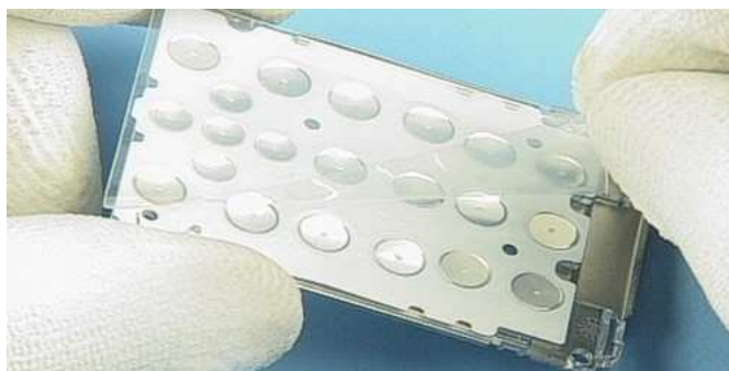
Before replacing the Light guide Assy remove the protection foil.
