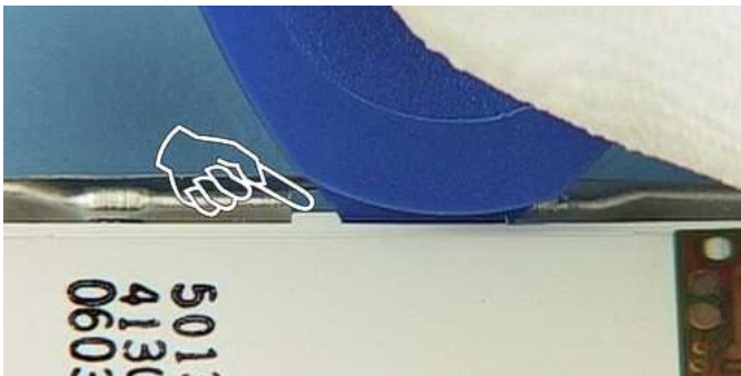
Use SRT-6 to separate the LCD-Module from UI-Shield.
