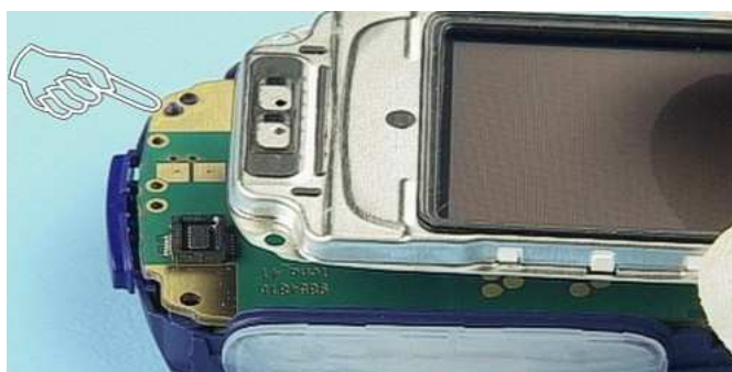
The last guiding pin is used for positioning the UI-Shield Assy.
