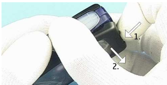
Press the C-Cover Lock before pulling the C-Cover.
