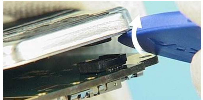
Open the LCD Connector with SRT-6 carefully.
