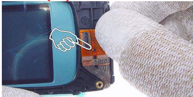
21.) Place the Board-to-Board connector into its compartment. Note the guide pin.
