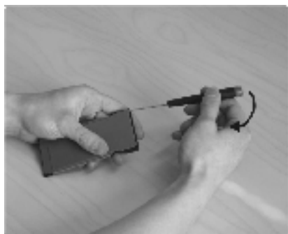
Fig. 8 : Open Bottom Cover subassembly
