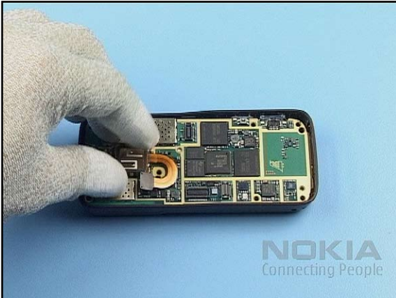
19. Insert the MAIN CAMERA into its housing...
