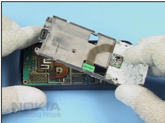
28. Remove the UI FRAME with the UI MODULE from the B-COVER.
