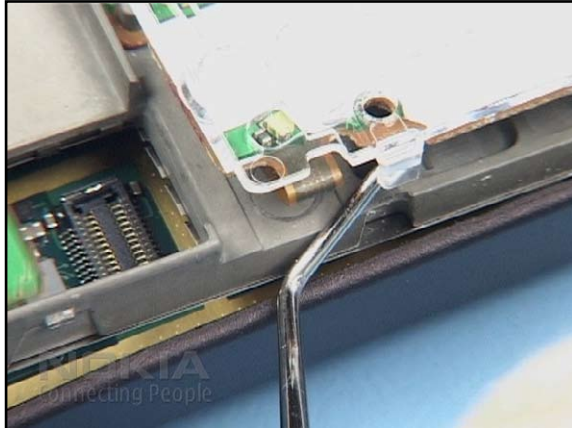
26. Lift the UI FRAME a bit and unsnap the LIGHT GUIDE.
