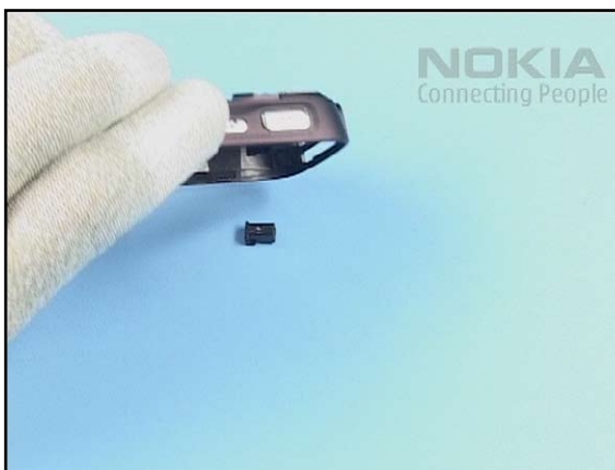
46. The DC-JACK drops out easily when turning the B-COVER.
