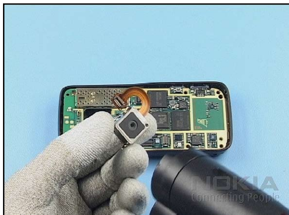
18. and the MAIN CAMERA with compressed air.
