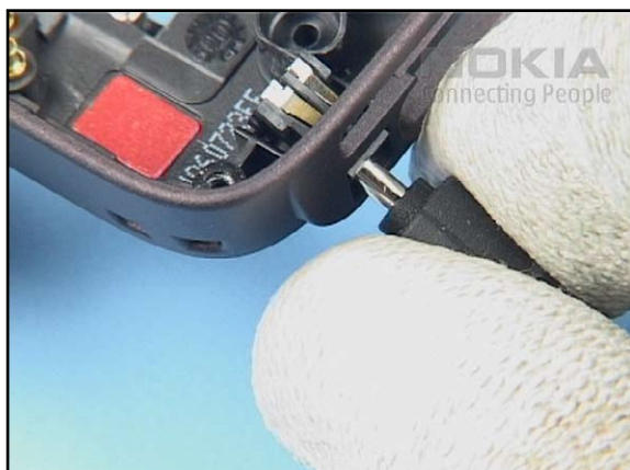
45. Use the DC plug to release the DC-JACK.
